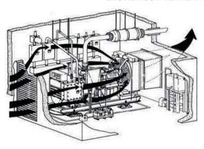
Engine room ventilation can be estimated by the following formulas, assuming  $100^\circ$  F  $(38^\circ$  C) ambient air temperature:
